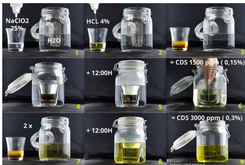
Fig. 50: Preparation of CDS using hydrochloric acid as the activator
